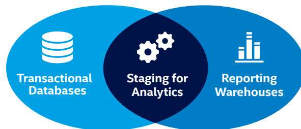
Figure 5. The retail banking logical data model consists of several transactional databases, a staging area for analytics (often called the enterprise data warehouse or EDW), and reporting warehouses.
